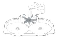
**Q4** Reassemble the left and right cleaning discs and self-cleaning assembly back into the cleaning tray in turn, and then reinstall them at the bottom of base station after drying.
