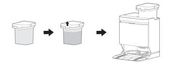
**O2** To empty the dirty water, remove the Waste water tank on the left, open the cover, and pour out the water.
